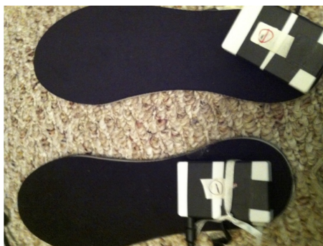
Fig. 2: Sensor system inside the sole of shoes.
